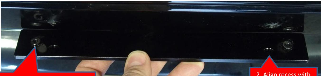
1. Align Tag Delete. The raised threaded holes go inside the existing bumper holes.
