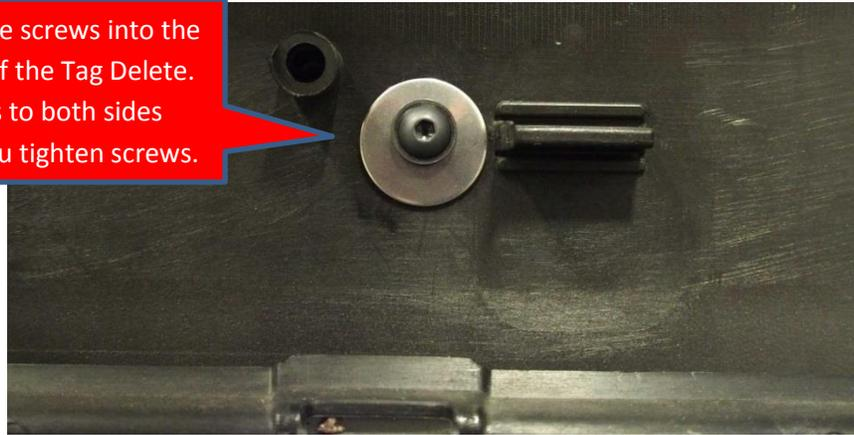
5. Tighten Allen screw with included 2.5mm allen key while holding the tag delete to make sure raised area stays in the holes on the bumper.
